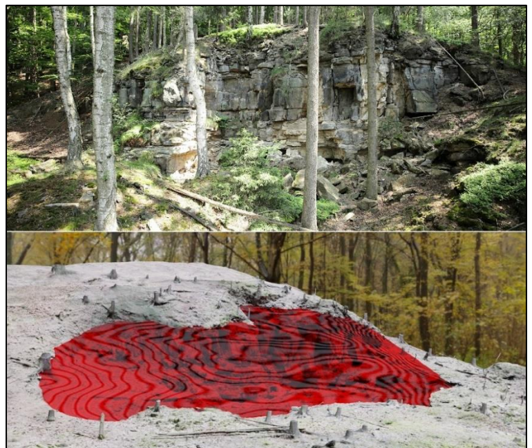
Fig. 4. A whetstone quarry near Podskalí in the Elbe River Canyon with unstable rock wall; the extracted mass of sandstones with a volume about 1200 m 3 is marked on the 3D model by red color (photo and model J. Horák).
